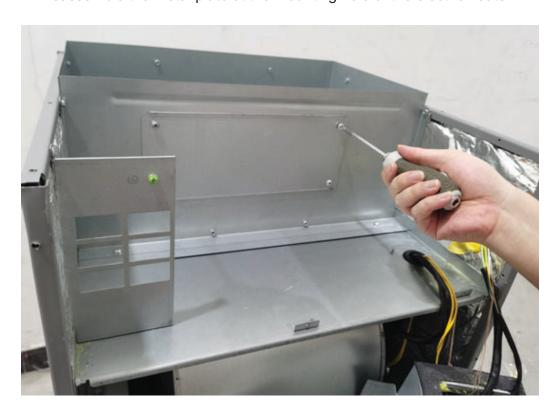
5. Install the electric heater to the metal plate position which disassembled in step 4. (Notes: There are two holes circled below which are used to fasten the electric heater bracket during installation).
